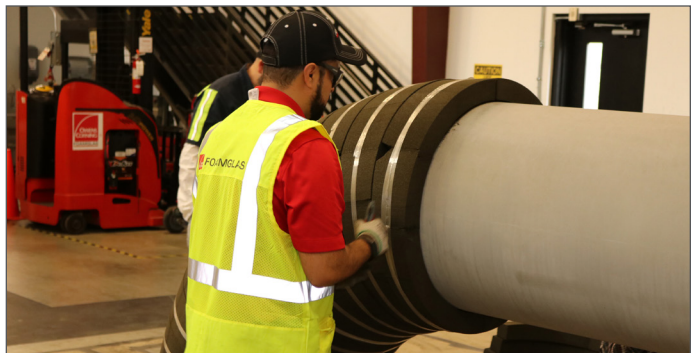
Mitered Elbows: Narrow pieces are more fragile and likely to damage in transport. The mitered system also creates more joints and reduces thermal protection.
